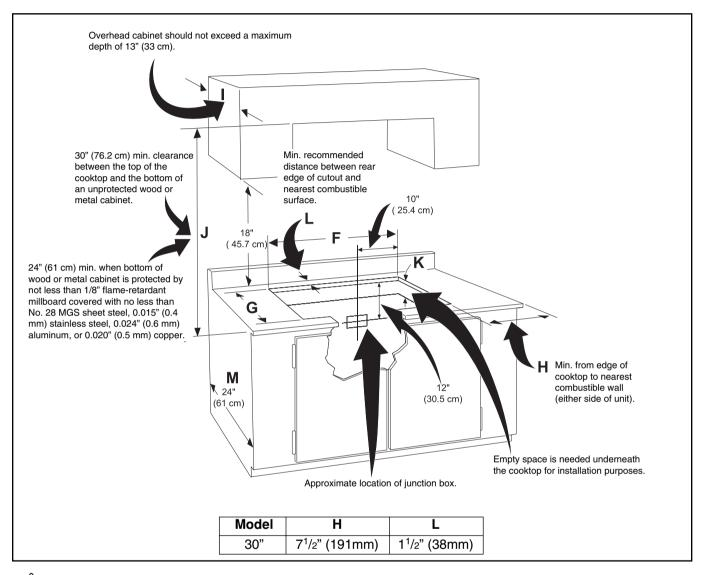
CAUTION: To eliminate the risk of burns or fire by reaching over heated surfaces, cabinet storage space located above the cooktop should be avoided. If cabinet storage is provided, risk can be reduced by installing a range hood that projects horizontally a minimum of 5" (12.7 cm) beyond the face of the cabinets.
